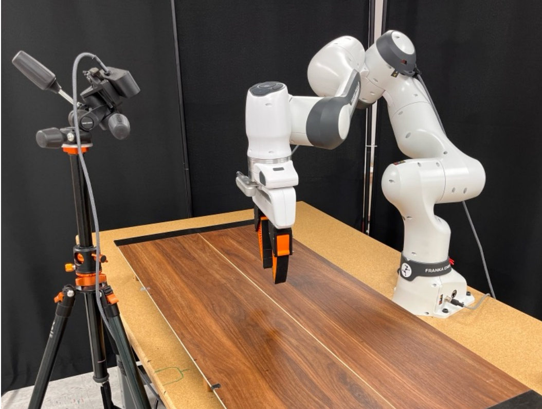
Figure 1: Our hardware experiment setup, we use a Franka Research 3 robot, with a UMI gripper. The RealSense D435 wrist camera, and Zed mini 2i third person camera are placed as shown.
